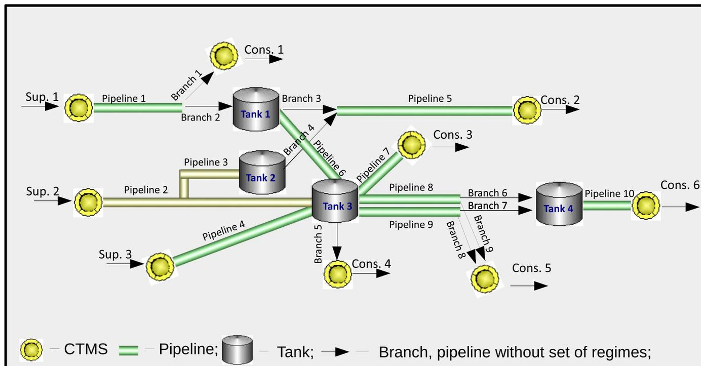
Fig. 1. Scheme of the branched oil pipeline system. Cons. = consumer; and Sup. = supplier.
